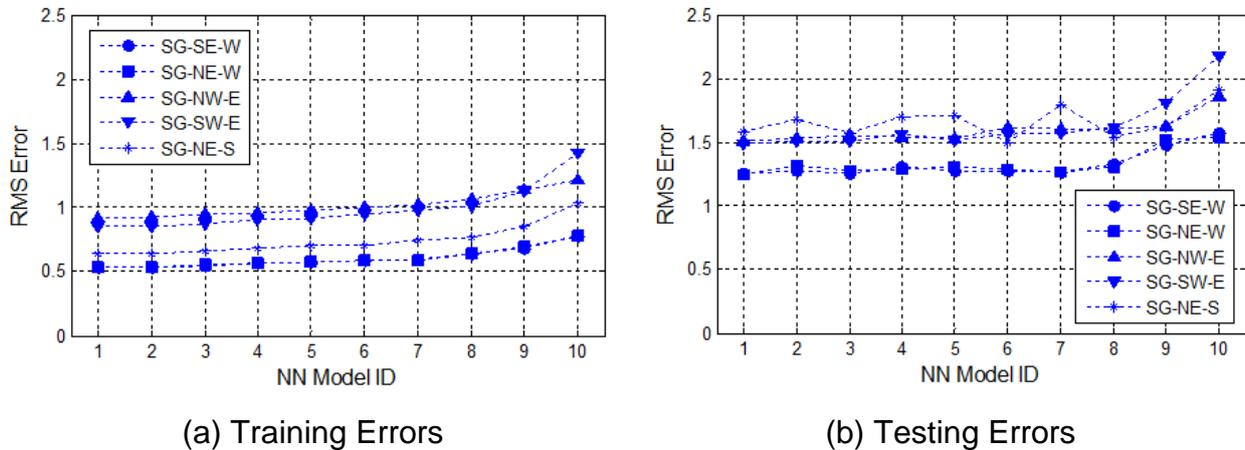
Fig 7. Training and Testing Errors of Neural Networks Based Strain Prediction Models
