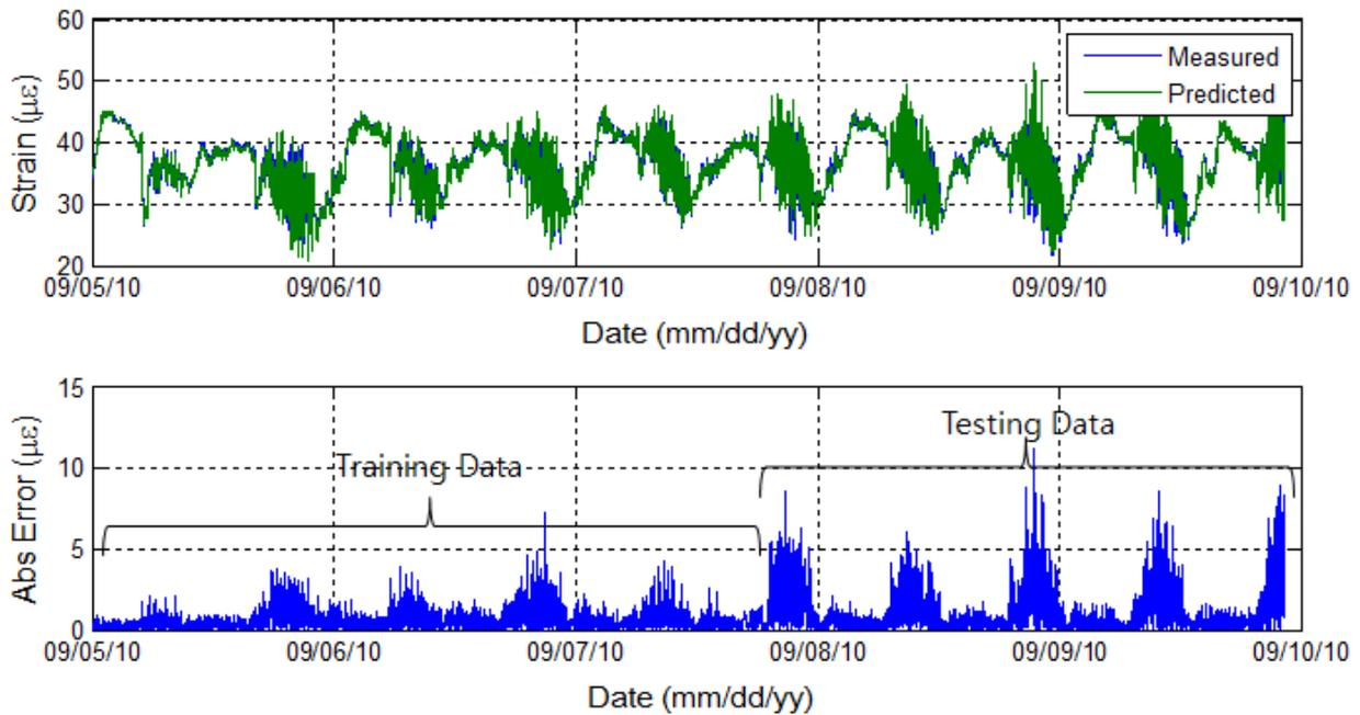
Fig. 8 Measured and Predicted Strain Time Series and Errors between Two Data
