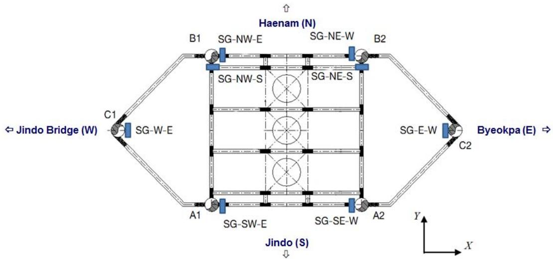
Fig. 3 Installation Locations of Strain Gauges
