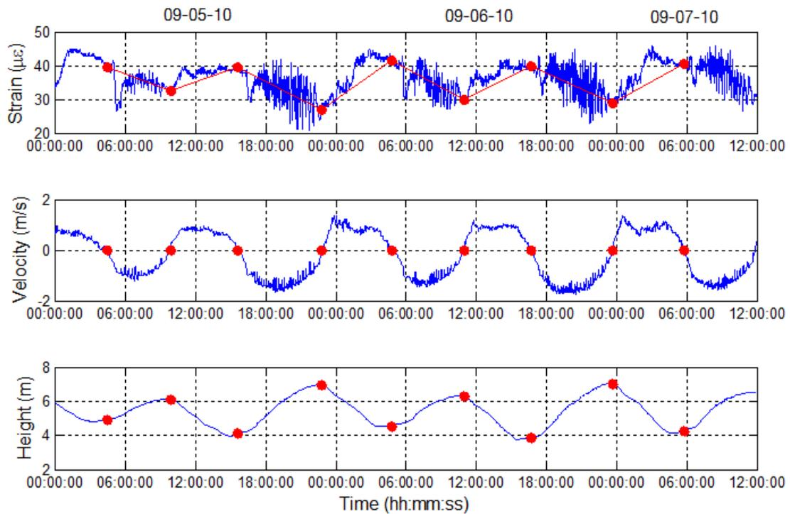
Fig. 4 Measured strain data from September 5 to 7, 2010 (● denotes the still water condition)
