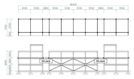
Fig.1Planof the test specimen and Test setup
