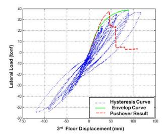
Fig.9Comparison of Analytical and Experimental Results
