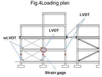
Fig.5 Measurement Sensor Location
