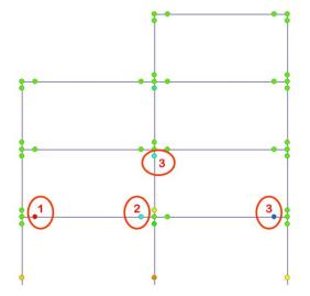
Fig.10Sequence of Plastic hinge Development
