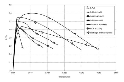
Fig. 9 Predicted stress-strain relationships for the first group specimens
