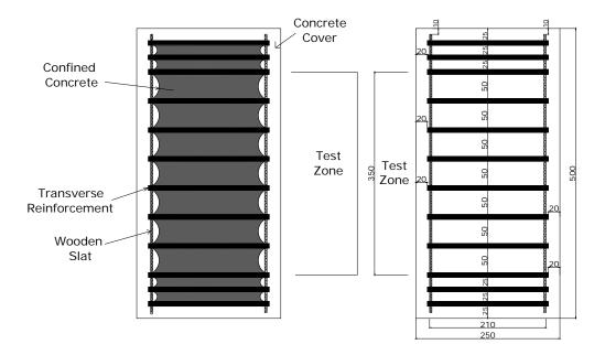
Fig. 2 Transverse reinforcement detailing (all dimensions are in mm)
