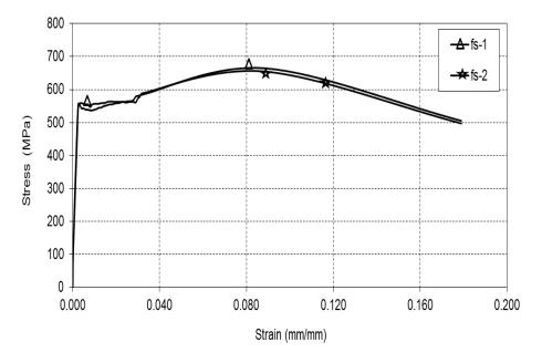
Fig. 1 Stress-strain relationships of transverse reinforcement
