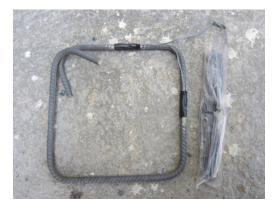
Fig. 5 Transverse reinforcement with strain gauges
