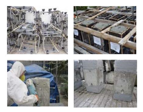
Fig. 3 Specimen preparation
