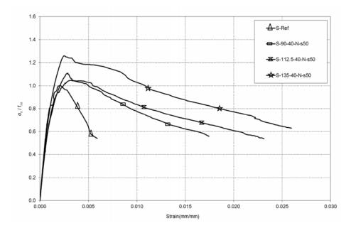
Fig. 6 Stress – strain relationships of the first group specimens
