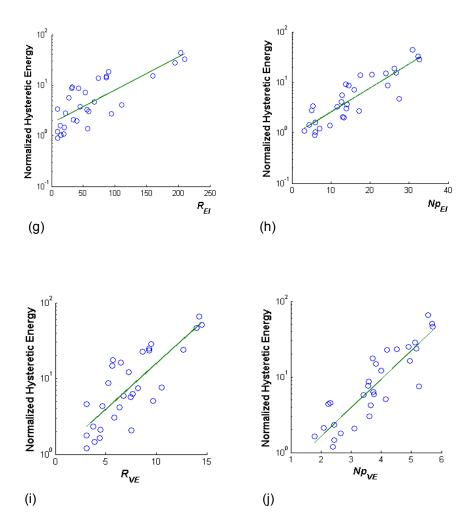
Fig. 3. Prediction of normalized hysteretic energy for the steel frame F4 with T<sub>1</sub>=0.90s  $(Sa(T_1)=1000 \text{ cm/s}^2)$  for: (a) *PGA*; (b) *PGV*; (c) *I<sub>D</sub>*; (d) *t<sub>D</sub>*; (e) *R<sub>Sa</sub>*; (f) *N<sub>pSa</sub>*; (g) *R<sub>El</sub>*; (h)  $N_{pEl}$ ; (i) *R<sub>VE</sub>* and (j) *N<sub>pVE</sub>*
