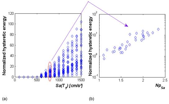
Fig. 2 (a) Incremental dynamic analysis scaling for  $Sa(T_1)$ ; (b) Relation between  $N_{pSa}$  and the normalized hysteretic energy at  $Sa(T_1)$ =800cm/s<sup>2</sup>
