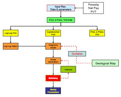
Fig. 3 Pressure transient analysis workflow (LAPI ITB, 2010)
