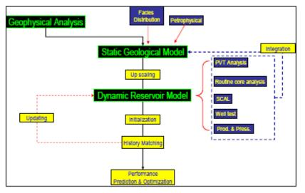
Fig. 4 Reservoir simulation workflow (LAPI ITB, 2010)
