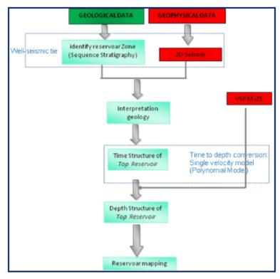
Fig. 1 Geophysical analysis workflow (LAPI ITB, 2010)
