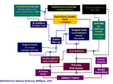
Fig. 2 Flow chart of geological analysis methodology (LAPI ITB, 2010)
