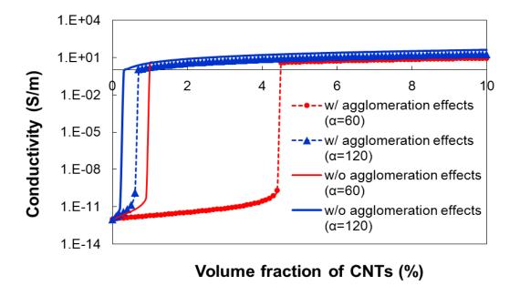
Figure 1. The predicted electrical conductivity of the nanocomposites with respect to the aspect ratio ( $\alpha$ ) and agglomeration of CNT
