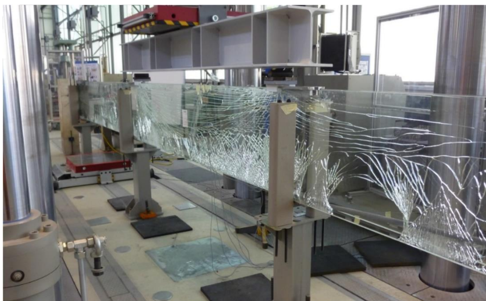
Fig. 1 Crack pattern of a 9.0 m post-tensioned glass beam. Engelmann (2016)
