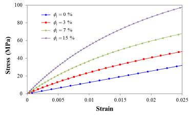
Figure 1. The predicted stress-strain behaviors composites with respect to the volume fraction of carbon fiber
