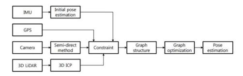
Fig. 1 Graph-based SLAM algorithm (developed by Prof. H. Myung (KAIST))
