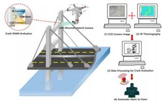
Fig. 2 Crack evaluation technique based on hybrid scanning image from CCD and IR cameras (developed by Prof. Y.K. An (Sejong Univ.))
