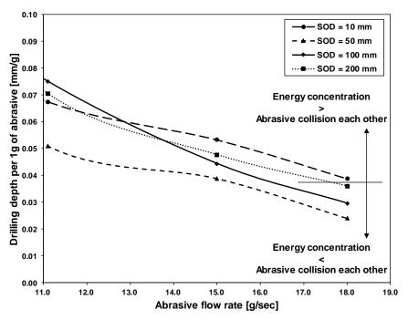
Fig. 3 Unit mass of abrasive effect on the drilling depth
