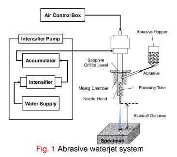
Drilling tests were performed by changing standoff distance (SOD), and abrasive flow rate (AFR) in the same granite specimen. Experimental conditions consisted of 5 cases of abrasive flow rate (i.e. 5.6, 7.5, 11.1, 15.0, and 18.0 g/sec) and 4 cases of standoff distance (i.e. 10, 50, 100, and 200 mm) combination (Table 2). It was total 20 cases. In all cases, the exposure time was set to 60 seconds. After drilling was completed, the depth, width, and removal volume of each hole were measured.
