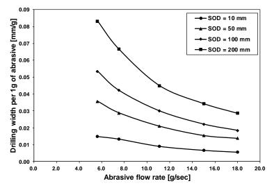
Fig. 4 Unit mass of abrasive effect on the drilling width
