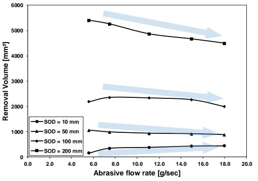
Fig. 2 Effect of abrasive flow rate on the removal volume
