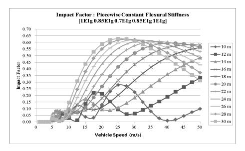
Fig. 3 Impact Factor : Piecewise constant flexural stiffness (cracked bridge) [1El<sub>g</sub> 0.85El<sub>g</sub> 0.7El<sub>g</sub> 0.85El<sub>g</sub> 1El<sub>g</sub>]
