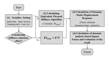
Fig. 2 The MATLAB program's flowchart
