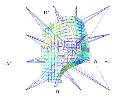
Fig.2 collapsing procedure of the double layer grid due to support loss with an abnormal live load
