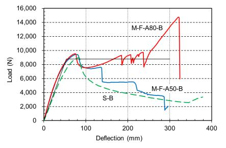
Fig. 4 Load-Deflection depending on support conditions
