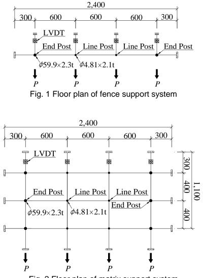
Fig. 2 Floor plan of matrix support system
