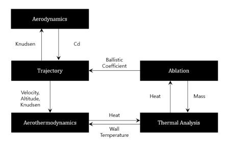
Fig. 1 Schematic program modules[Sim 2010]
