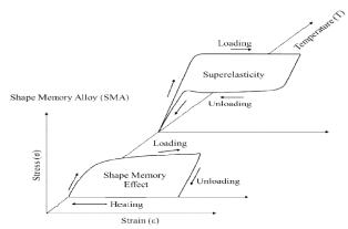
Fig. 1 Superelastic SMA materials
