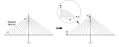
Fig. 1 Simulation of cable rupture (Park et al. 2007)
