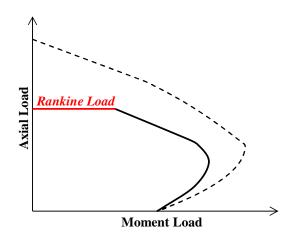
Fig. 1 Main concept of proposed P-M interaction curve model of a RC column
