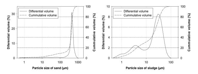
Figure 1 Particle size distribution of sand and sludge
