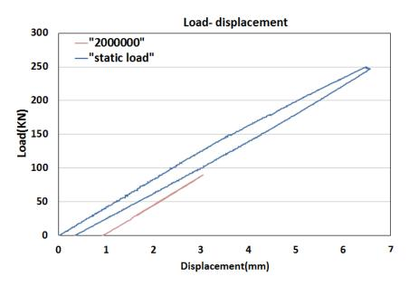
Fig. 5 Load- deflection curve (loading point of specimen)
