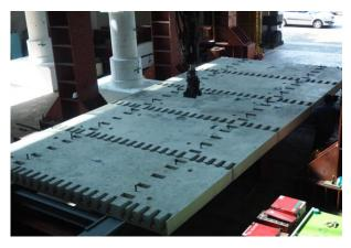
Fig. 1 Load tests of composite bridge using precast concrete deck
