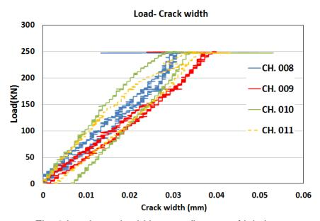
Fig. 6 Load- crack width curve (bottom of joint)
