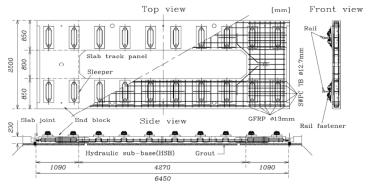
Fig. 1 Precast concrete slab track considered in this paper
