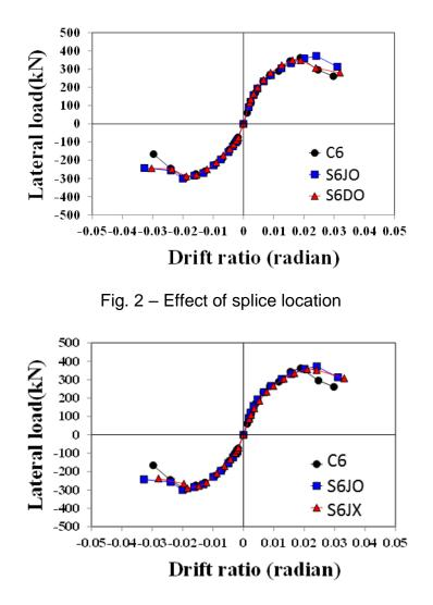
Fig. 3 – Effect of grouting
