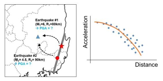
Fig. 1 Prediction of ground motions with respect to earthquake magnitude and epicentral distance
