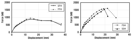
Fig. 2 Envelop of load-displacement (Left: SFH and FFH, Right: SSH and FSH)
