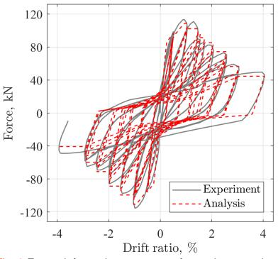
Fig. 2 Force-deformation response of experiment and analysis
