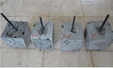
Fig. 5. Pullout test.
