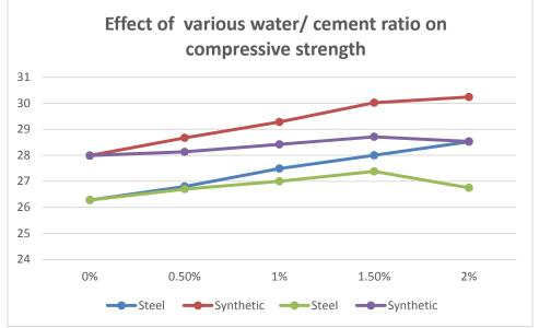
Fig. 4. Effect of various water/ cement ratio on compressive strength with various fiber
