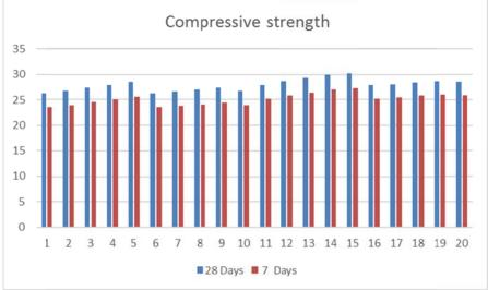
Fig. 1. Compressive strength of 7-days and 28-days concrete
