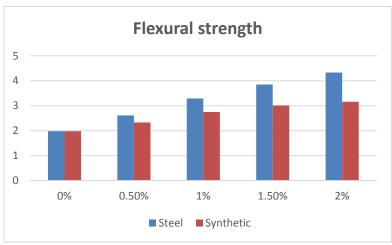
Fig. 3. Flexural strength of 28-days concrete
