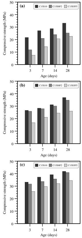
Fig. 2 Strengths development of hardened paste with different curing schemes: (a) T20, (b) T30 and (c) T40
