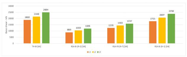
Fig. 6 The comparison base shear of fixed base and base-isolated
