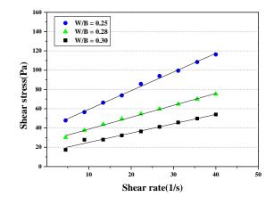
Fig. 2 Results of measuring the rheological properties of mixtures with different W/B ratios
