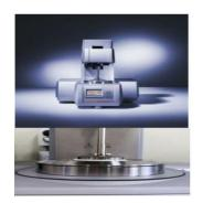
Fig. 1 Rheometer used for cement paste rheology measurements
