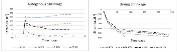
Fig.3: Autogenous Shrinkage and Drying Shrinkage
