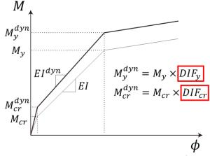
Fig.1 Dynamic moment-curvature relationship of the RC section
