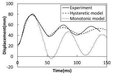
Fig.3 Displacement time history at mid span of RC1
