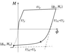
Fig. 2 Unloading branch in hysteretic moment-curvature relationship
