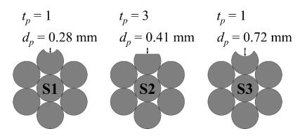
Fig. 2. Test specimens of corroded strands.
