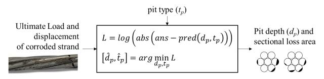
Fig. 3. Inference method to evaluate the corrosion configurations.
