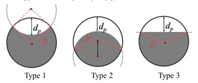
Fig. 1. Pit shapes for FE analysis (Jeon et al. 2019).
