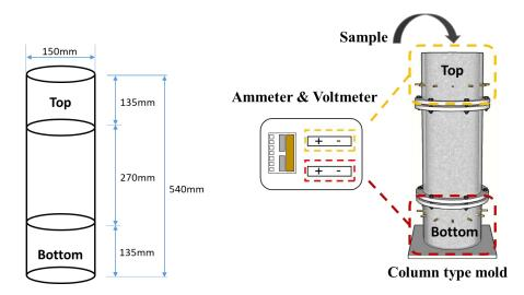
Fig. 2 Electrical resistivity measurement mold for evaluation of concrete segregation
