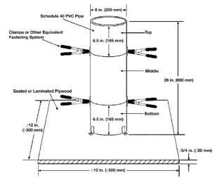
Fig. 1 Column type mold for evaluation of concrete static segregation
