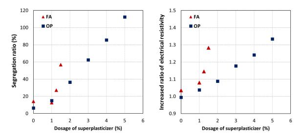
Fig. 5 (a) Increased ratio of electrical resistivity by dosage of superplasticizer (b) Segregation ratio by dosage of superplasticizer
