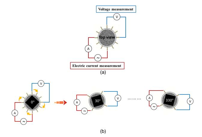
Fig. 3 (a) Electrical resistivity measurement system using electrode square configuration (b) Twelve rotating system for averaged electrical resistivity
