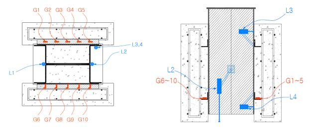
Fig. 1 Push-out specimen and measurement plan
