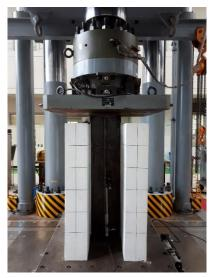
Fig. 2 Push-out test set up with UTM
