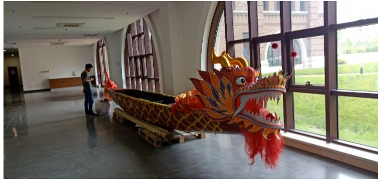
Fig.9 Full-scale concrete dragon boat
