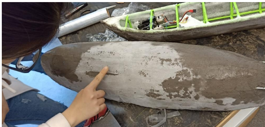
Fig.5 Fabrication of concrete dragon boat model
