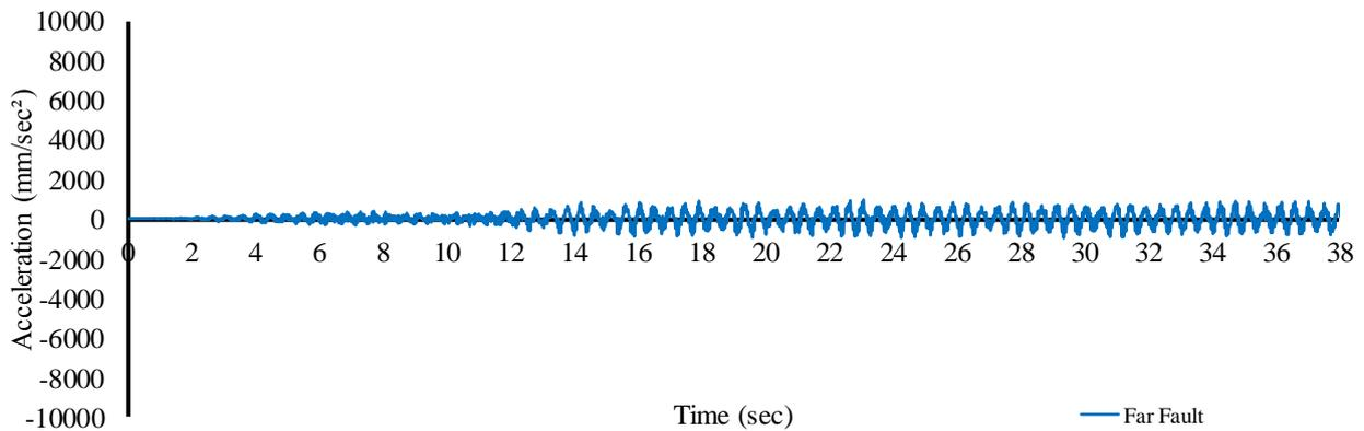
Fig. 11 Seismic accelerations on Point 11348 during middle fault earthquake for structure without NSC.
